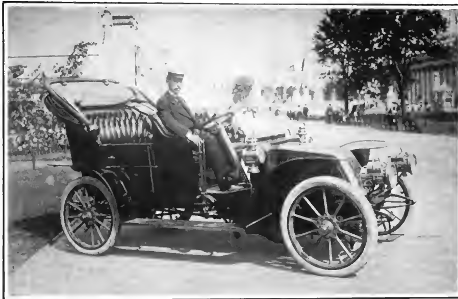
LATEST MODEL RENAULT DOUBLE PHAETON WITH SIDE ENTRANCE AND HOOD AND EQUIPPED WITH THE NEW STYLE OF RADIATOR.
